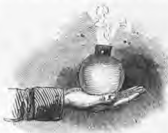
FIG. 98. Red-hot Iron Ball on the palm of the Hand, protected by some powdered charcoal.
