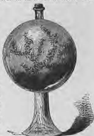
Fig. 141. Engraver's Globe, with Arborescent Precipitate of Silver. The globe, of course, must be entirely filled with the solution.
