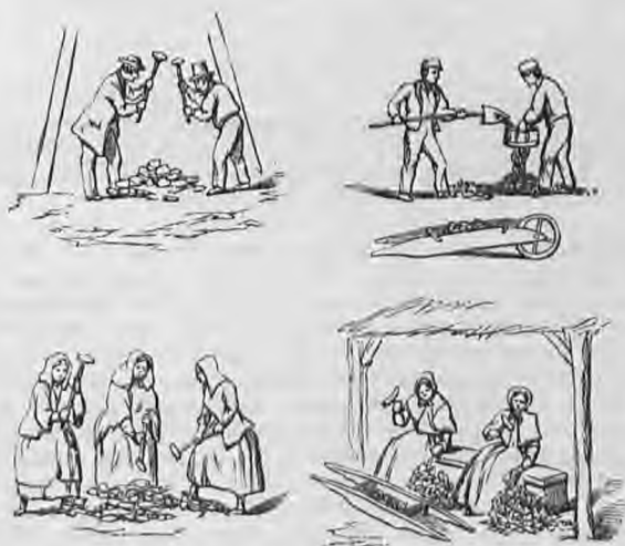
Fig. 100. Ragging, Spalling, Riddling, and Cobbing the Copper Ore.
