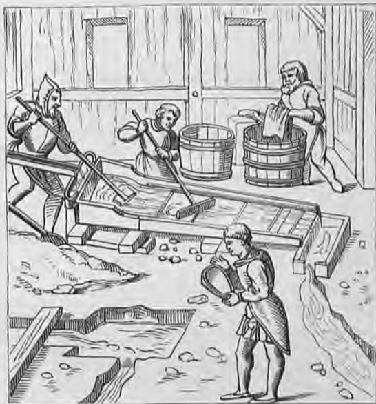
Fig. 153. The "Nicking Buddle." (Agricola.)
