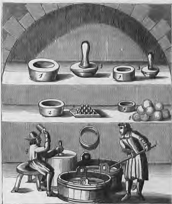
Fig. 136. "1 and 3. Copel moulds or cases. 2 and 4. The copels that are made in them. 5. The copels as they are set upon one another. 6. The washed bone-ashes or char made into balls. 7. He that works the ashes. 8. He that strikes the copels into their moulds or cases." (Pettus.)
