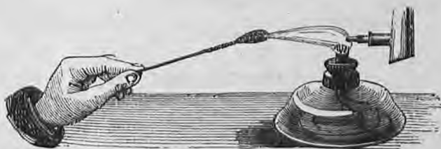
Fig. 245. Manganese Compound, fused on a loop of platinum wire with phosphate of soda and ammonia, which is sometimes called microcosmic salt.
