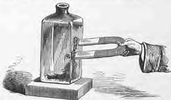
Fig. 218. Magnet drawing up the Magnetic Oxide of Iron (contained in Water) at the Side of the Bottle.
