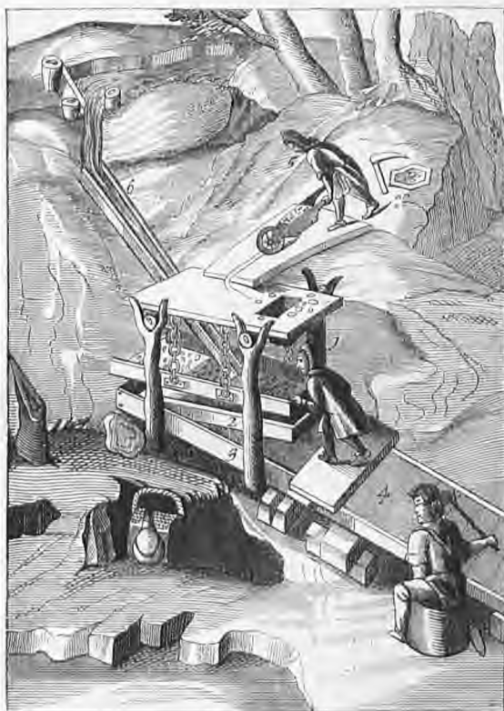
Fig. 105. Ancient Gold Washers (Pettus). "1. The man that worketh with the Rattar (or shaking sieve). 2. The middle floor, whereon that which goeth through the Rattar doth fall. 3. The lower floor, whereon that which cometh from the middle floor doth fall. 4. The plain receiver, called the hearth, of that which falls from both. 5. The person that stands on a board, and out of a wheelbarrow throws the matter or ear into the tunnel which guides it into the Rattar. 6. The channel in which water doth run into the Rattar."
