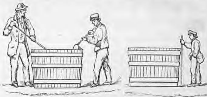
Fig. 177. Tossing and packing Tin Ores. (Henderson.)
