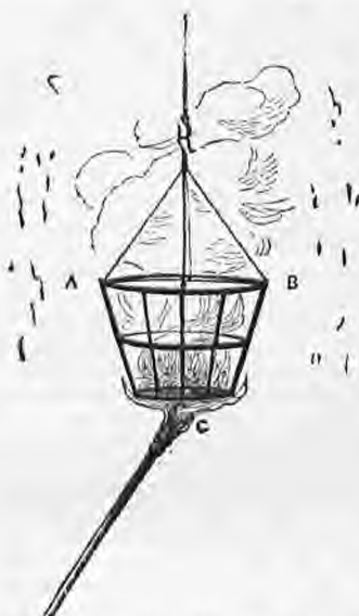
Fig. 264. A B. Iron-wire basket containing the zinc turnings, and having a very little tow at the bottom saturated with spirits of wine. C. The lighted torch for igniting the tow at bottom of the basket. The falling particles indicate the oxide of zinc.
