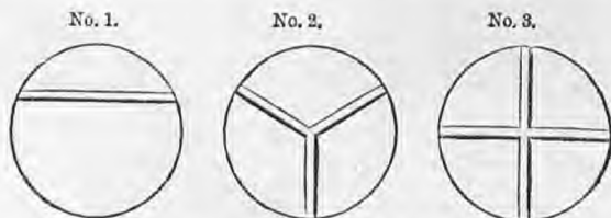
Fig. 34. Various Methods of dividing a Coal Pit Shaft for Ventilation and drawing Coals, &c.
