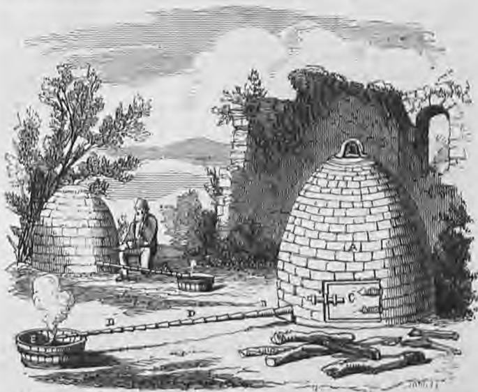
Fig. 91. Glauber's Method of procuring Acetic Acid by the destructive Distillation of Wood, copied from his "Miraculum Mundi." "A is the Furnace or oven, wherein the wood is char'd. B. The Cover of the Furnace. C. The door at which the coals are taken out. D. The Canes or Pipes wherein the sap or juices of the wood is condensed, and from thence runs into the receiver. E is the vessell or receiver into which the vinegar of wood runs."
