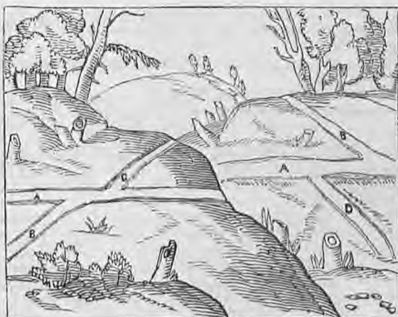
Fig. 161. A, chief vein. B, intersecting or cross vein. C, The other part of B, removed from its natural position (rapta). The further removal and alteration of the original position and continuity of the vein is shown to the right at D & E. (Agricola.)
