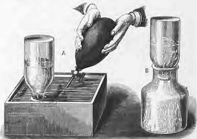
Fig. 60. A. Passing coal gas into a narrow-mouthed bottle in the pneumatic trough. B. Bottle half full of coal gas, and the remaining half water; the latter is falling out, and the air is taking its place.
