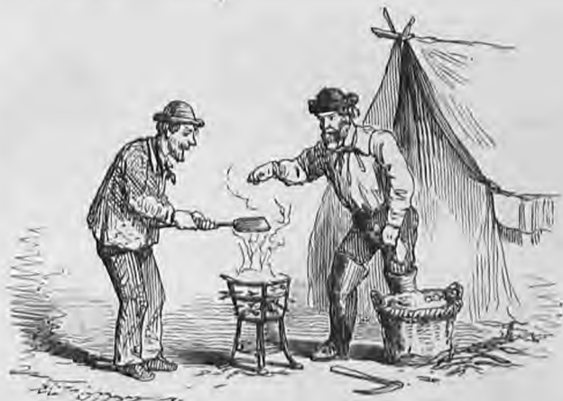
Fig. 116. Testing for Pyrites by the red-hot Shovel.
