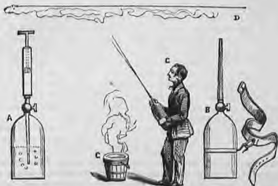
Fig. 172. A. Section of copper bottle with pipe, condensing pump, and stopcock. The bottle is half full of the alcoholic solution. B. Copper bottle ready for use, with the jet screwed on and attached to a leathern belt by a ring and hook. C. Pail of boiling water. D. Use of the copper bottle, from which the jet of alcohol escapes to the ceiling D, where a torch of tow dipped in spirits of wine is held for a few minutes, till it takes fire properly.
